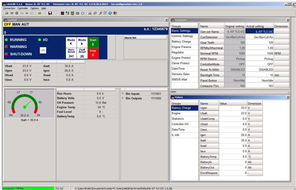
The screenshot displays the LiteEdit 5.1.2 software interface for an IL-NT TLC-DC controller. The main window is titled "Control" and shows the status "OFF MAN AUT" with a serial number "s.n.: 12345678". The status indicators include RUNNING (green), WARNING (red), and SHUT-DOWN (red). The control panel features buttons for Mode, Start, Horn Reset, Fault Reset, and Stop. A central gauge shows the battery current (Ibatt) at 30.0 A. The interface is divided into several sections:
