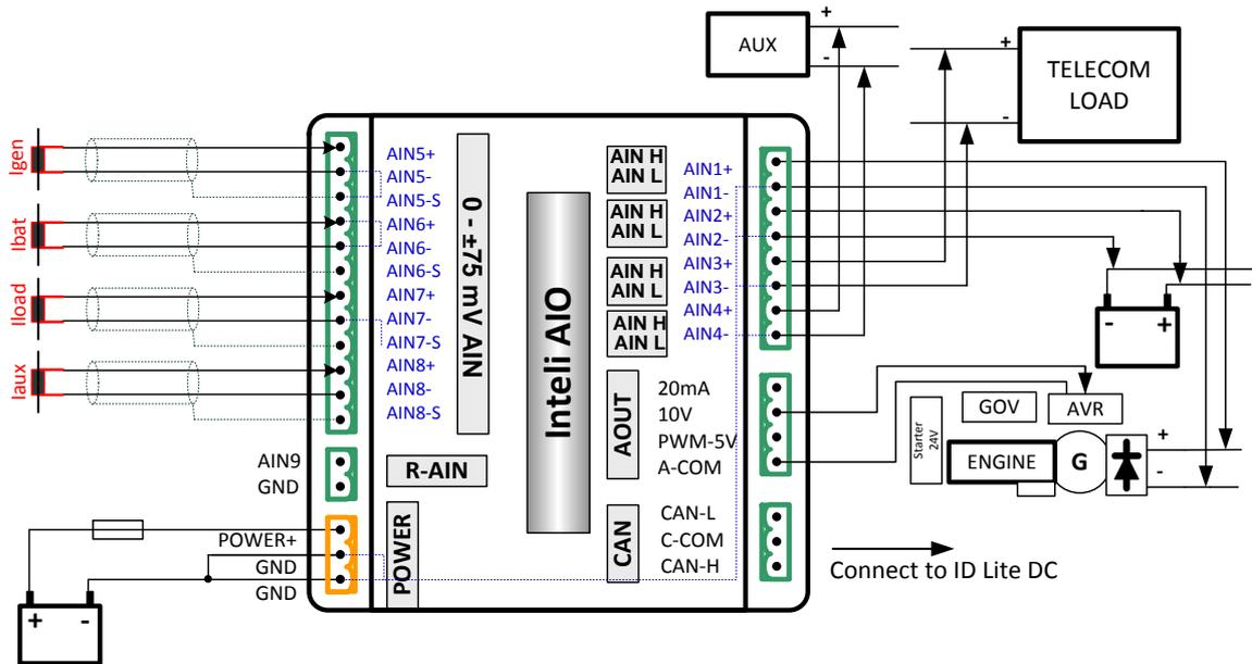
Modify default configuration according to actual project wiring – e.g. set corresponding Analog input as not used when not used.
