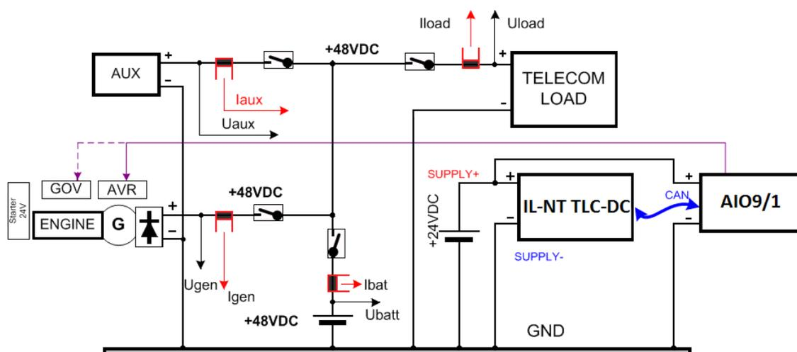
Example of wiring for nonstandard PLUS pole grounding IntelliLite Telecom DC and AIO9/1 module:
