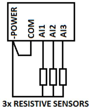
Standard connection of three resistive sensors to analog inputs.
