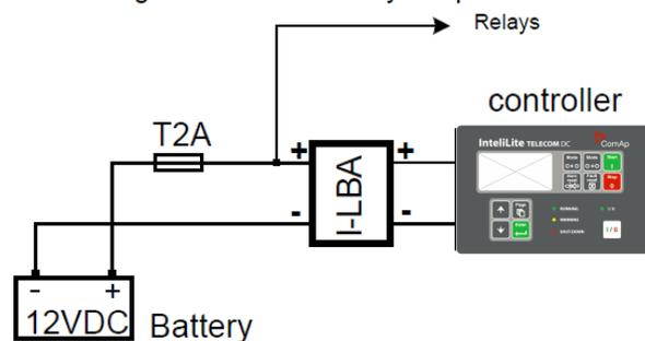
Connecting the external capacitor. The capacitor size depends on required time. It shall be approximately thousands of uF (microFarads). The capacitor size should be 5000 uF to withstand 150ms voltage dip under following conditions: Voltage before dip is 12 V, after 150 ms the voltage recovers to minimum allowed voltage i.e. 8 V.
