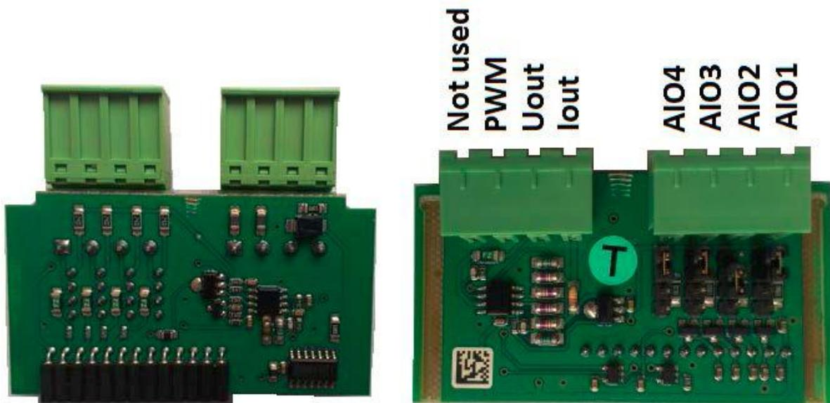
Type of analog input is selectable by jumper. Each analog input has own line of jumper position. The top position (closest to green connector on the pic above) is for resistive input, central position for voltage input and lowest position is for current input.
