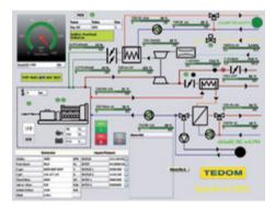
InteliMonitor is a free SCADA SW for visualization of data in process applications. It can be customized to create visualization of individual systems as well as producing automatically generated screens using the supplied templates.
