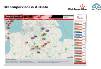
WebSupervisor is cloud-based system designed for monitoring and controlling ComAp controllers via the Internet. This system offers a number of beneficial features that help optimize revenue for machinery fleets, as each piece of equipment can be individually monitored for all important operation values.
