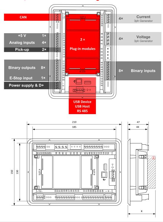
**Note:** The final depth of the controller depends on the selected plug-in module – it can vary between 41 mm and 56 mm. Mind also the size of connectors and cables (e.g. in case of RS232 connector, add about 60 mm more for standard RS232 connector and cable).
